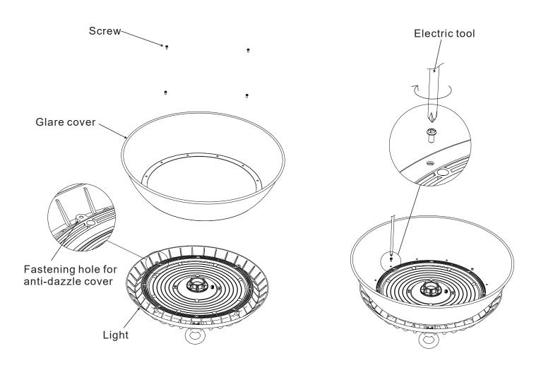
1. Align the hole of the anti-dazzle cover with the fixing hole of the radiator
